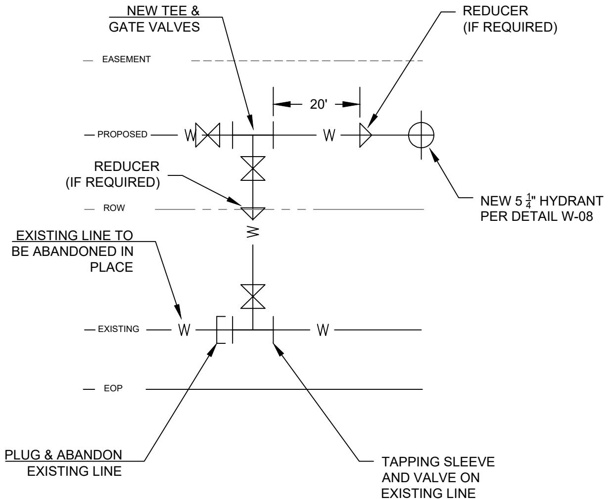
**END OF LINE CONNECTION DETAIL (WITH EASEMENT)**
