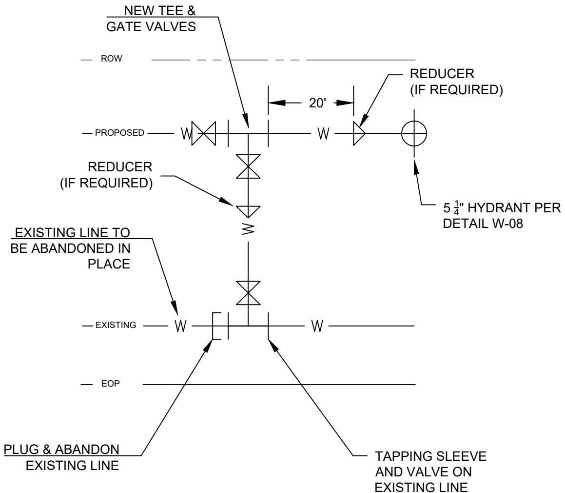
**END OF LINE CONNECTION DETAIL (NO EASEMENT)**
